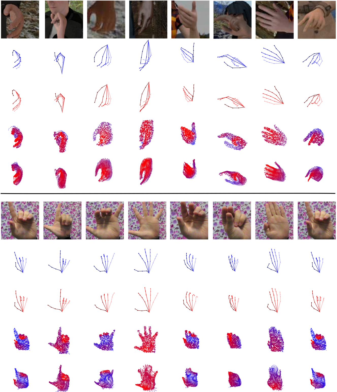
Figure 1: More examples on 3D pose estimation and point cloud reconstruction for RHD (top) and STB (bottom) dataset. From top to bottom: RGB images, ground-truth poses in blue, estimated poses from \mathbf{z}_{rgb} in red, ground-truth point clouds, reconstructed point clouds from \mathbf{z}_{rgb} . The color for point clouds decodes the depth information, closer points are more red and further points are more blue. Note that the ground-truth point clouds are not used for inference, it is shown here only for comparison purpose.
